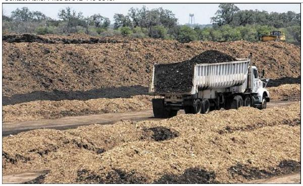
Piles of yard trimmings are mixed with sewage solids to create Dillo Dirt at the Hornsby Bend Biosolids Management facility. The city of Austin has been losing, typically, between \$400,000 and \$500,000 a year on slow sales, and officials are considering hiring a private waste hauler to reduce the pileup around the plant. AMERICAN-STATESMAN 2011
